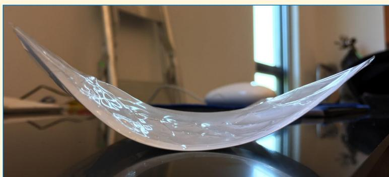
(Left) The air bubbles and curving show the extent that PO film shrank mid-print and pulled on its backing.
