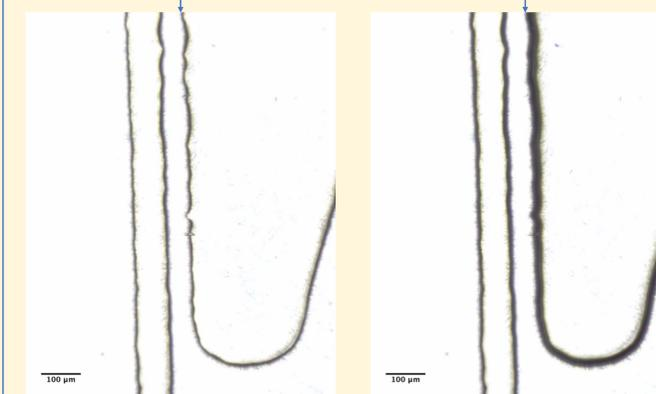
(Left) An unpressurized plunger < 100 μm from a channel. (Right) The same plunger with pressure applied. The bolder outline is from a shift out of focus due to upwards elastic deformation of the plunger.
