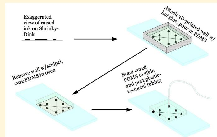
As seen in the top-left corner of the diagram, the design actually has a distinct height at the microscale which will actually create a negative PDMS mold when the latter is made solid through curing.
